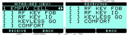
3. To receive the **RF KEY ID** signal, you must be at **up to 20 meters** from the car now when the key is brought to it. The car's mirrors will open and [+] **RF KEY ID** will appear on the device screen.
