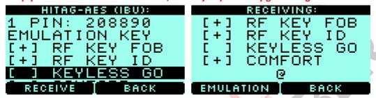
• To receive the **COMFORT** signal – **ONLY** approach the car, if the car is equipped with this function, the signal will be received and recorded in the device.
